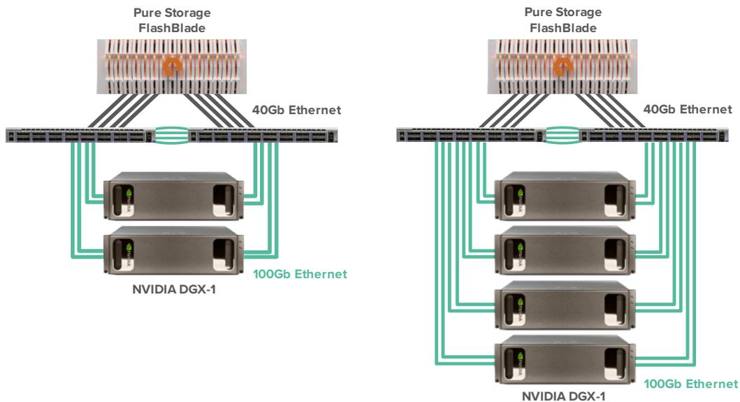
FIGURE 2. AIRI Mini and AIRI system architectures
