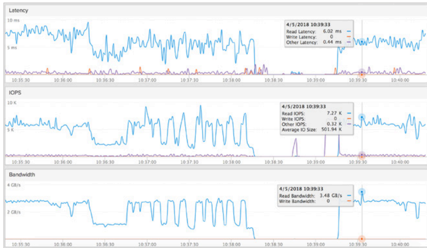
FIGURE 7. Screenshot taken from the FlashBlade UI while training a ResNet-50 model. The storage bandwidth, shown in the bottom graph, indicates an aggregate demand of nearly 3.5 GB/s. The brief dip in bandwidth indicates the input pipeline is filled with images waiting on GPUs to process.
