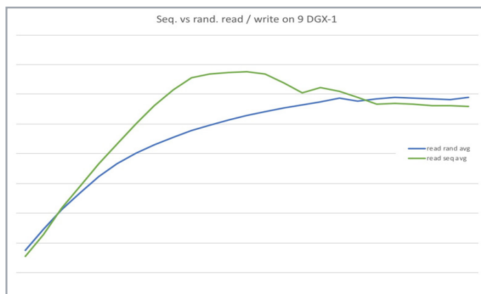
Figure 15: Sequential vs Random Read throughput with fio benchmark
