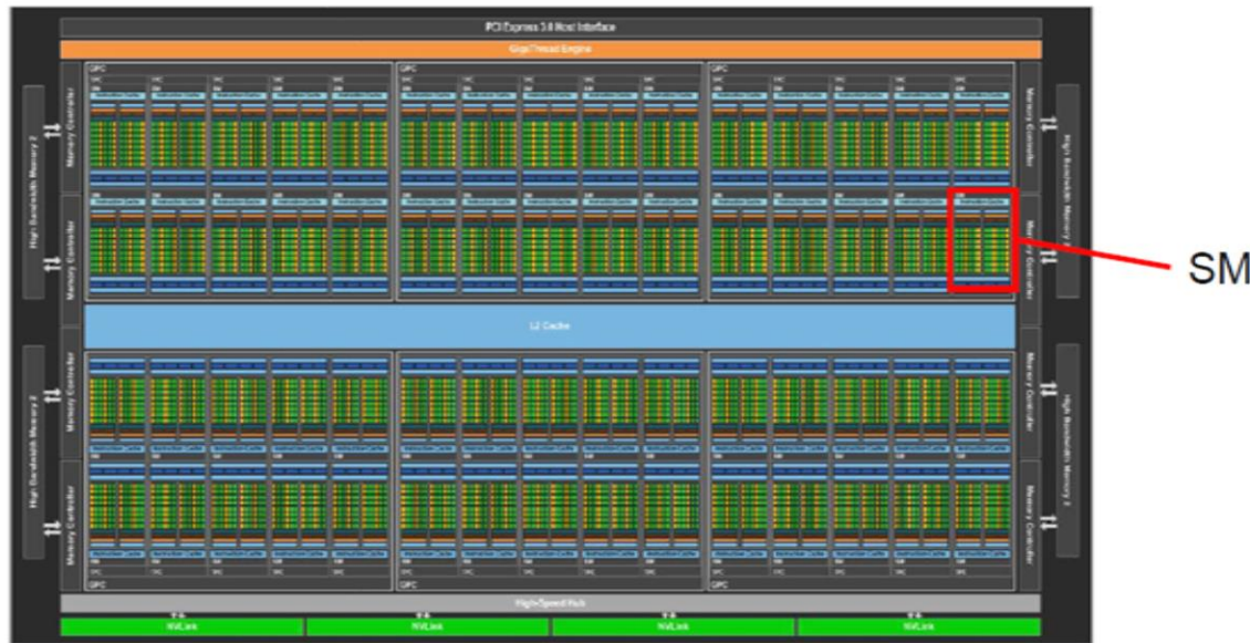
Tesla P100 Layout: 56 SMs, 3584 CUDA cores
