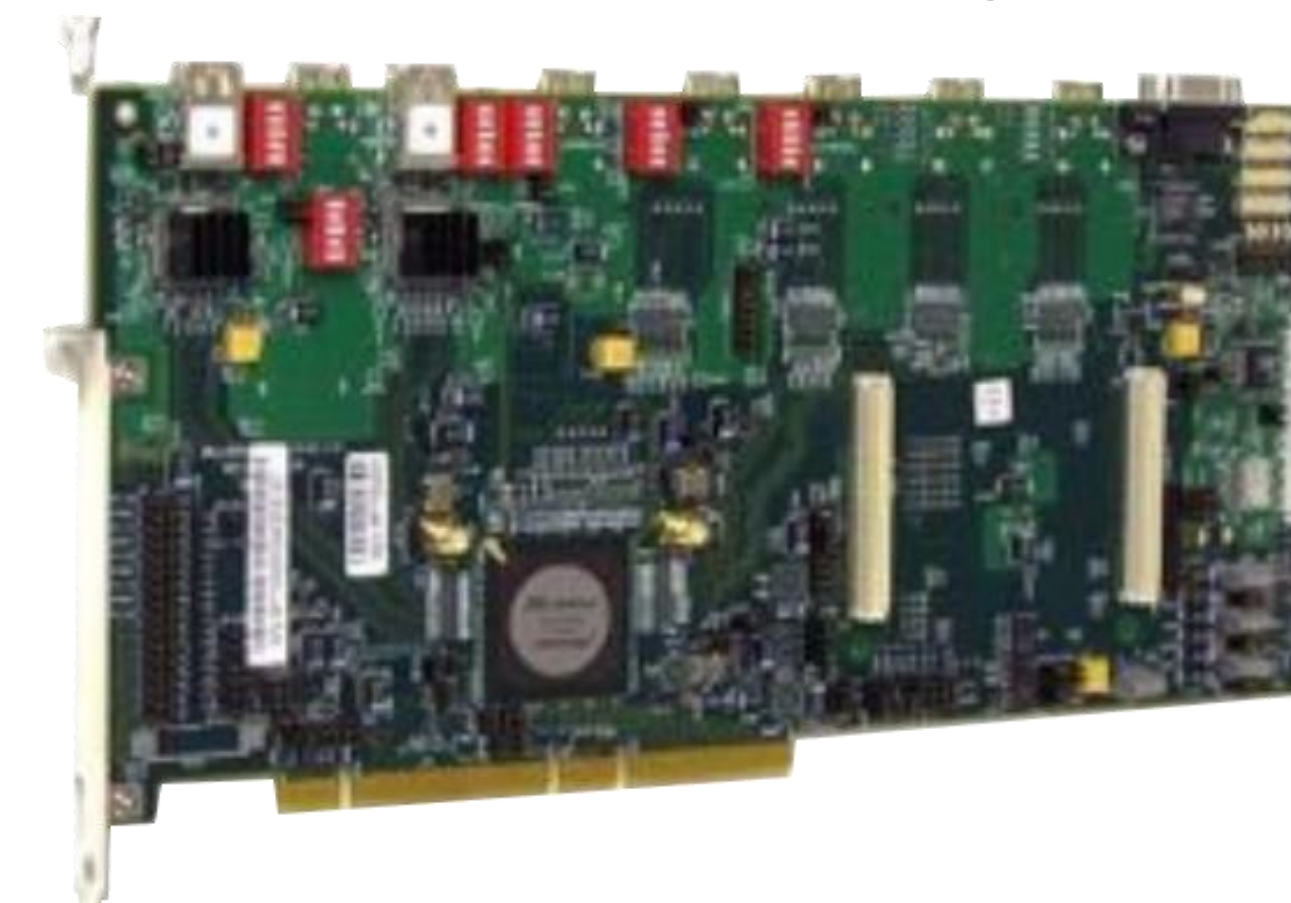
2001 InfiniBridge 10g IB HCA - Mellanox First Host Channel Adapter (HCA)
