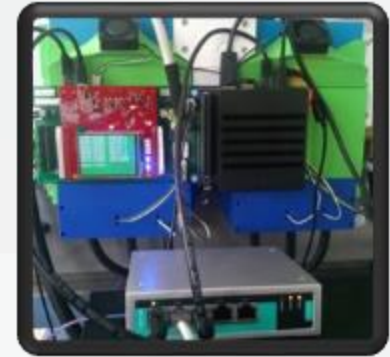
Dual three-phase power inverter Integrated platform for AI Extendable with additional modules using Ethernet
